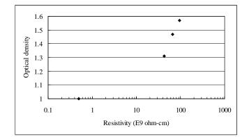
Figure 5. Relation between the resistivity of the ink and the O.D of the solid pattern
