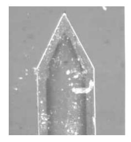
Figure 3. Magnification of the ink-guide; Thickness 0.1mm; Maximum width 0.7mm; Top degree : 50 degrees.
