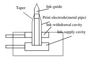
Figure 2. Cross-sectional view of the print head
